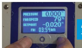
Figure 2 Menu driven zero calibration.
