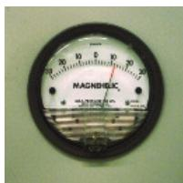
Once in service, air spaces will need to be monitored with suitable pressure sensors, so that the air pressure can be corrected as necessary on a continuous basis (left).
