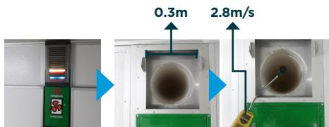
$$\text{Cross Section Area} = \pi r^2 = 3.14 \times \left(\frac{0.3}{2}\right)^2 \approx 0.07 \text{m}^2$$
