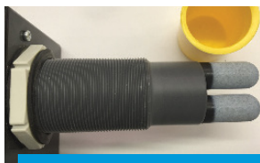
Figure 2 The photograph above shows typical CO 2 sensors in a setter, protected by sensor protection caps. If the caps become clogged with dust or condensation, the sensor will give an artificially high reading.
